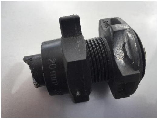
Philmac (PP) tank fitting failure in 50% hydrogen peroxide
